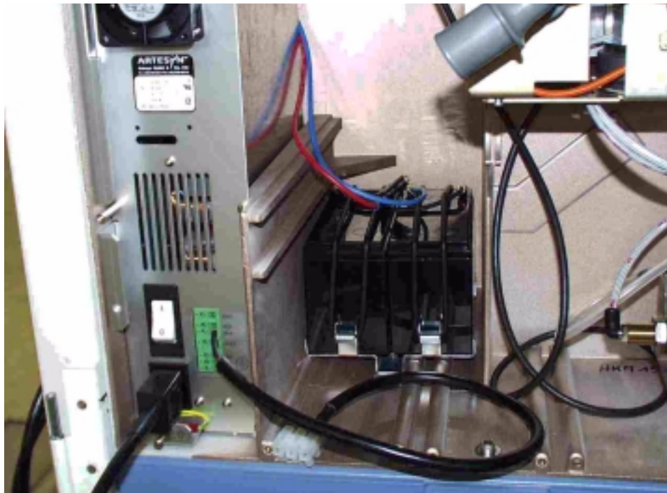
Fig. 48: Installed power supply unit 8601765, external battery pack 8601764 as of version "Ver04"
