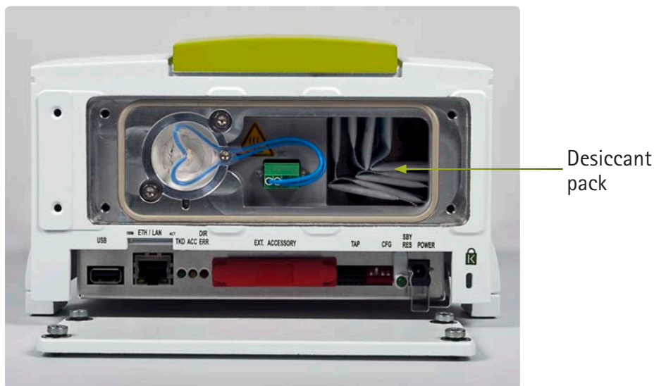
Figure 38. Replacing the desiccant
