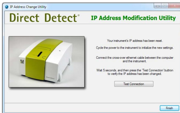
Figure 25. Testing the connection
