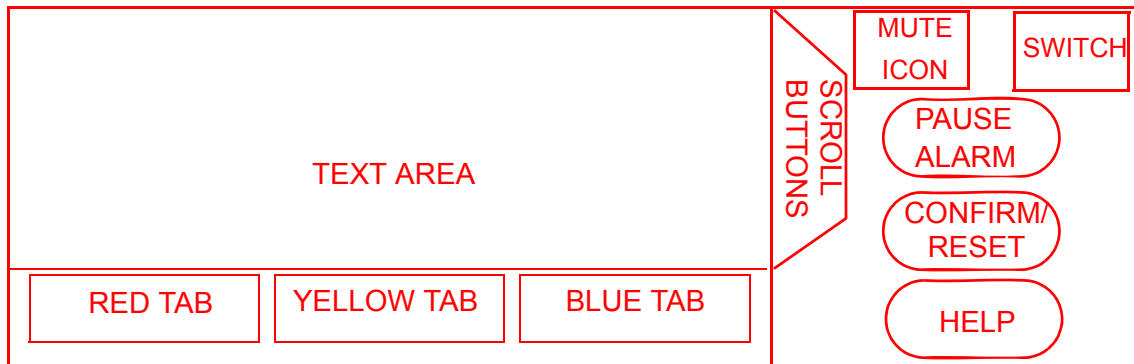
Figure 1-8. Alarm/Information Messages Area
