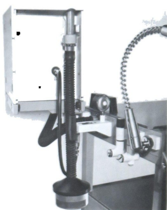
Fig. 13 Rear view of Ventilog attached to Tiberius 19 showing the anaesthetic filler attached to the exhaust gas nozzle
