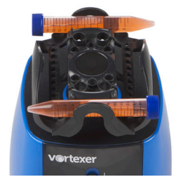
15 mL conical tubes x 2 (horizontally mounted)
