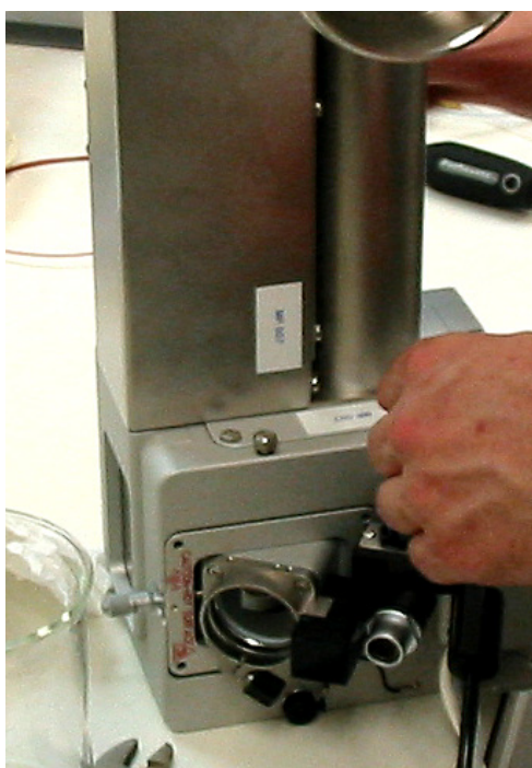
Figure 58. FAIMS interface and Ion Max source housing removed from the mass spectrometer
