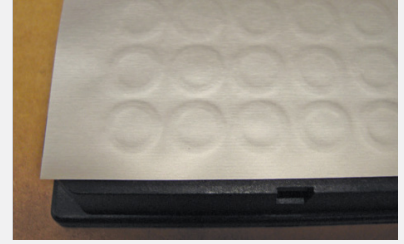
Fig. 9. Impressions should have uniform width around individual wells and across entire plate.
