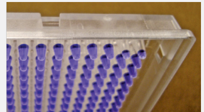
Fig. 11. Examine sample volumes after cycling. In this demo, corner wells were poorly sealed to demonstrate sample evaporation.
