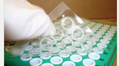
Fig. 10. Uniform and complete circles demonstrate good sealing.
