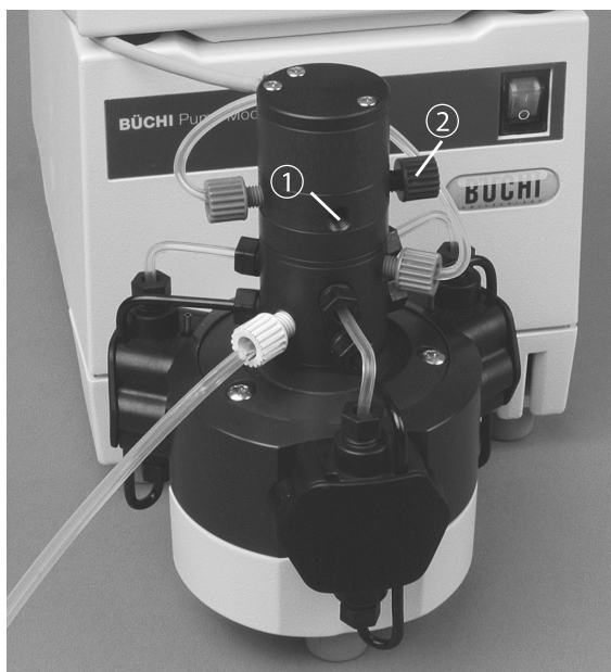
Fig. 5.13: Pump head with connected pressure tubing
