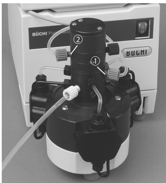
Fig. 5.12: Installing the suction tubing
