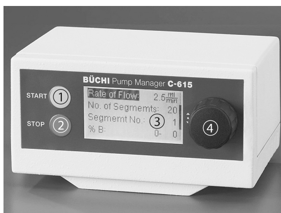
Fig. 6.2: Control arrangement on the Pump Manager
