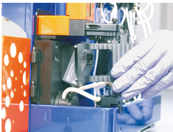
Figure 7.21: Dismantle the washing station.
