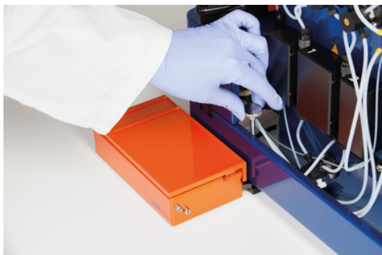
Figure 2.9: Secure the MACS MiniSampler Plus.
