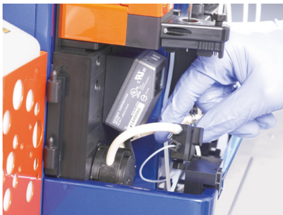
Figure 7.23: The draining tube is attached.
