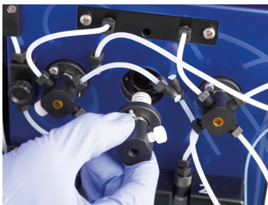
Figure 7.13: Detach the valve.
