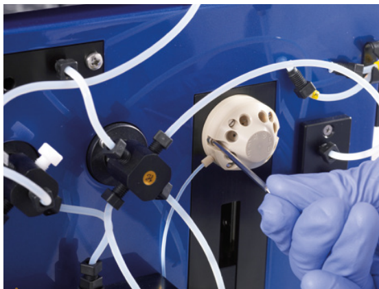
Figure 7.17: Unscrewing the dilutor valve's socket screws.
