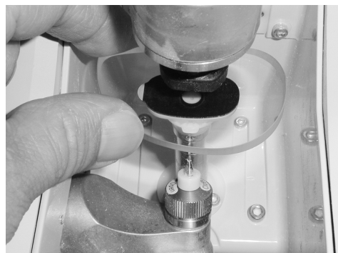
Set a lens to the cup holder with the lens top surface facing back.
