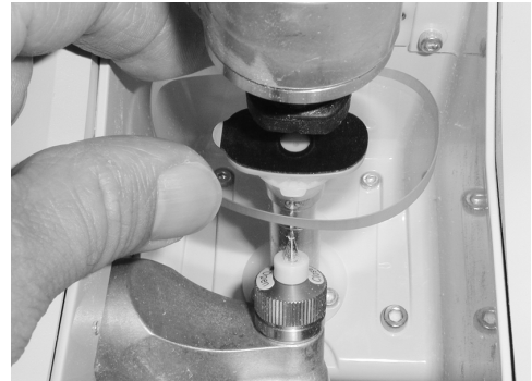
Set a lens to the cup holder with the lens top surface facing back.
