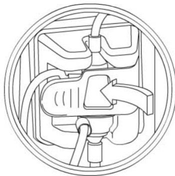
Figure Deaeration chamber
