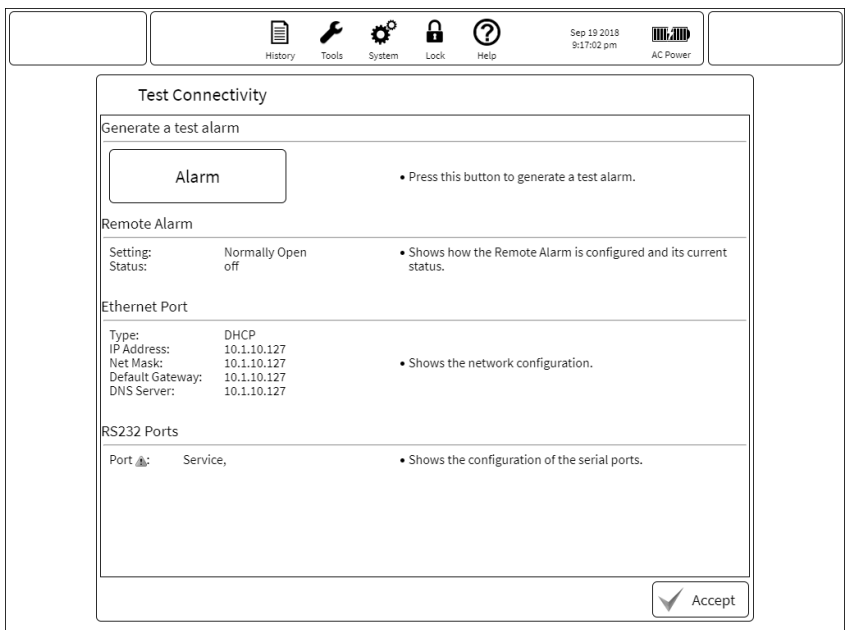
Figure Test connectivity window
