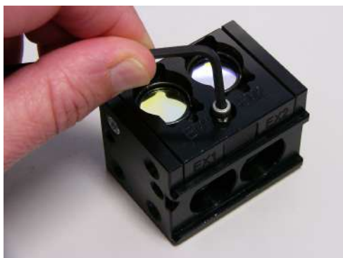
Remove the screw from the filter cube
