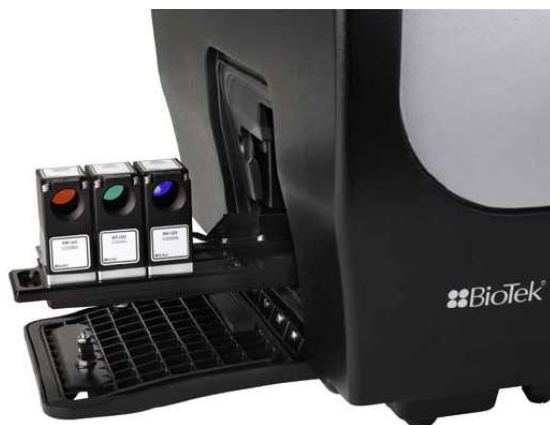
LED cubes and imaging filter cubes installed in positions 1, 2, and 3
