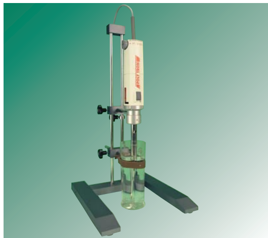
POLYTRON® PT 2100 with stand PT-ST 2101, dispersing aggregate and dispersing vessel
