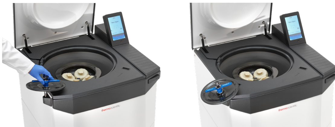
Figure 29: Using the Auto-Lock rotor lid holder
