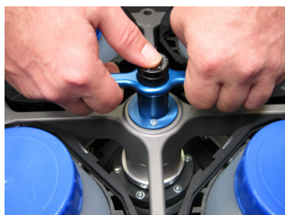
Figure 25: Holding the rotor during removal
