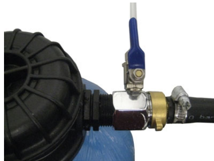
Figure 12: Open water drain (to replace the cartridge)
