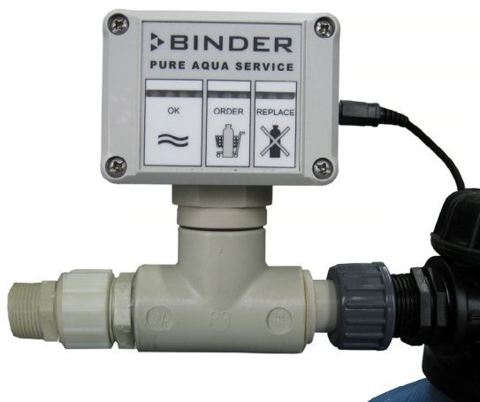
Figure 6: Measuring equipment connected to cartridge and mains unit
