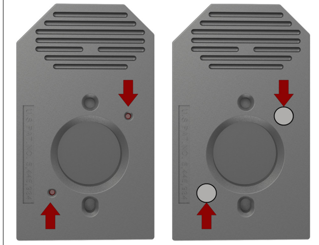
Figure 38 Applying Tough-Spots to array cartridge septa
