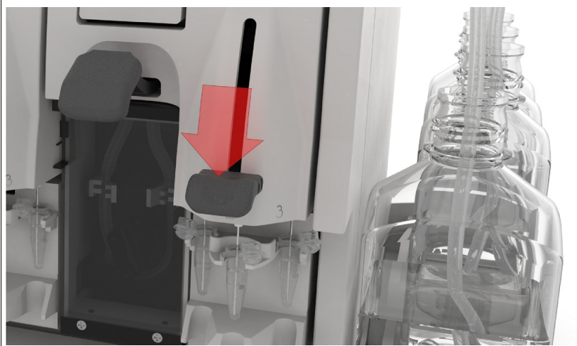
Figure 24 Press down on the needle levers to start the bleach protocol
