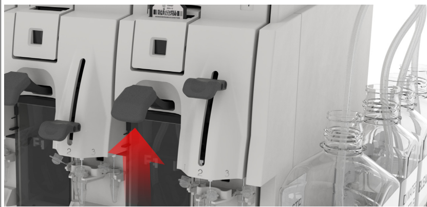
Figure 16 Flip the cartridge lever up to engage the cartridge septa needles into the septa, as shown.
