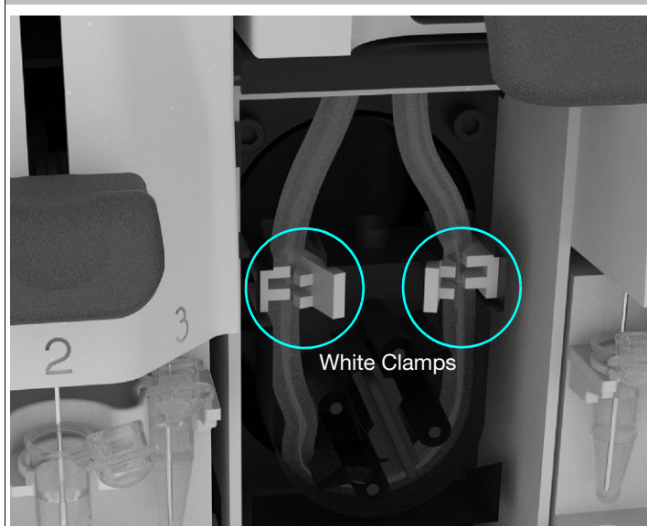
Figure 27 Releasing the peristaltic tubing
