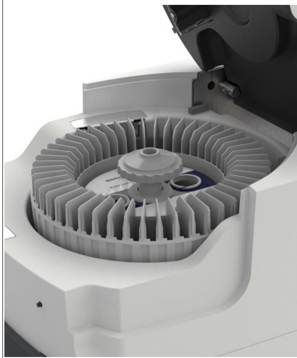
Figure 41 Inserting and turning the carousel. The carousel must be seated and flush with the housing.
