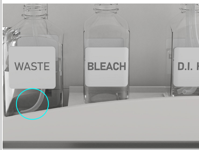
Figure 25 Immerse the three wash and water lines in the DI water bottle. Note: The waste line remains in the waste bottle.
