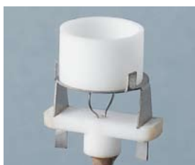
Sample carrier with Al 2 O 3 sample crucible
