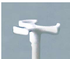
Standard Al 2 O 3 Sample carrier for corrosive gases
