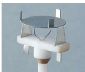
Sample carrier with Platine ® thermocouple
