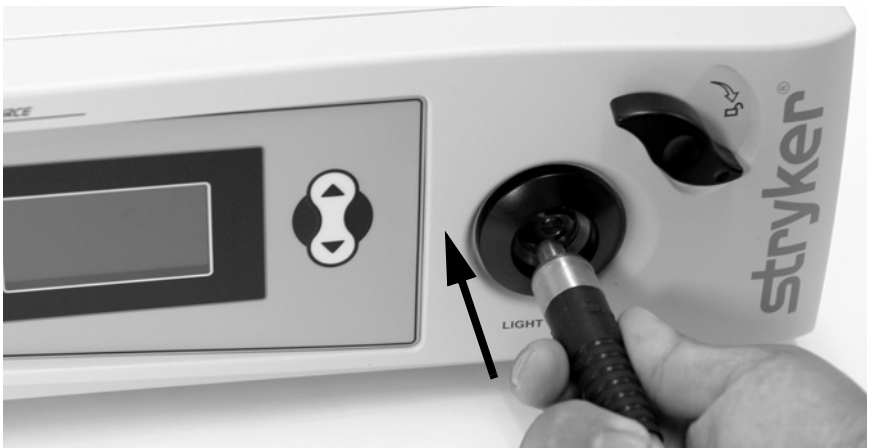
Figure 4 Inserting the light cable into the cable port
