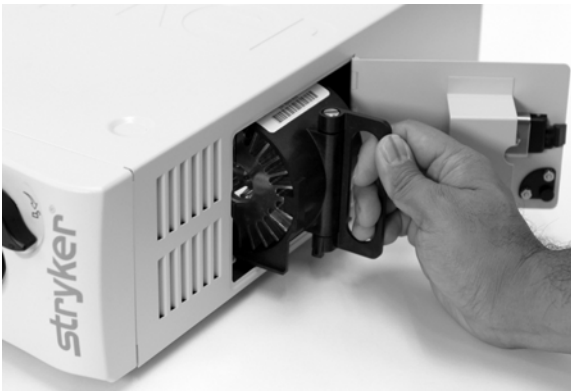
Figure 6 Removing the bulb module
