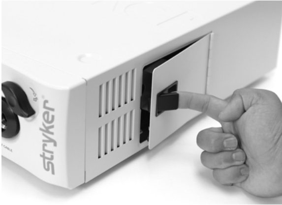
Figure 5 Opening the bulb door
