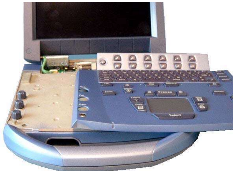
Figure 7.3 Control Panel Removal
