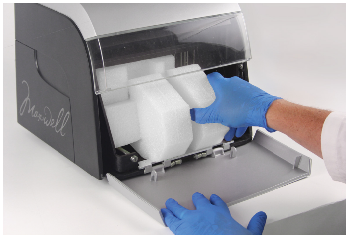
Figure 7. Removing the two foam pieces from inside the instrument.
