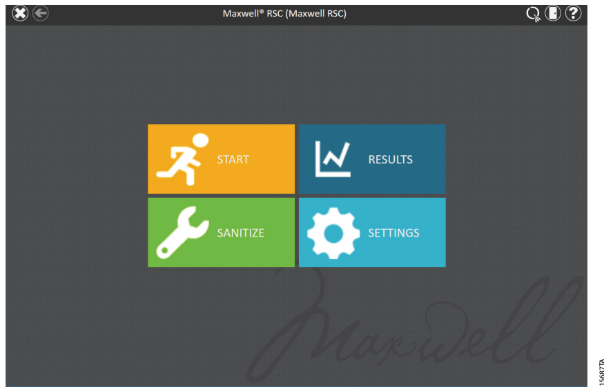
Figure 62. Maxwell® RSC 'Home' screen. Selecting Results opens the Maxwell® RSC 'Results' screen from which extraction reports from all method runs can be viewed.
