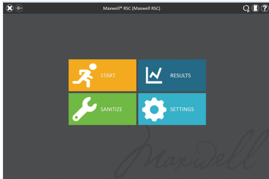
Figure 65. 'Home' screen. Selecting the Sanitize button begins the process for UV treatment of the Maxwell® RSC Instrument.
