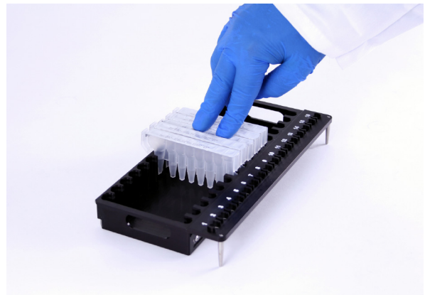
Figure 45. Placing the cartridges in the Deck Tray and pressing firmly to snap in place.
