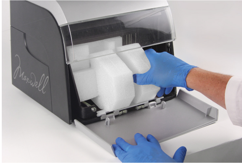
Figure 69. Placement of die cut foam in the Maxwell® RSC.
