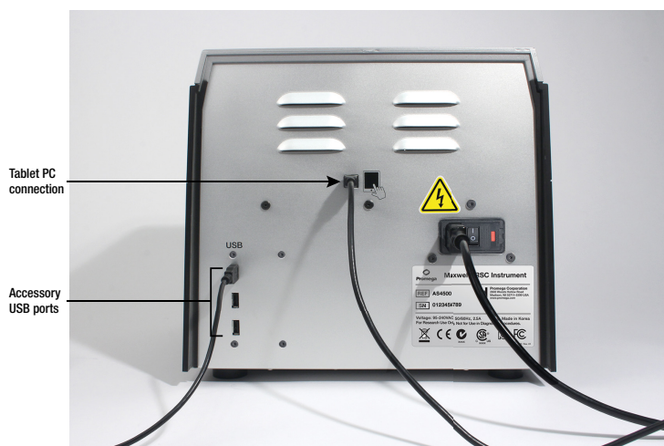
Figure 3. Rear of the Maxwell® RSC Instrument. The rear of the instrument showing the On/Off switch, power cable connector and USB communication port for the Tablet PC and the 3-port USB hub for accessories such as the Quantus™ Fluorometer.
