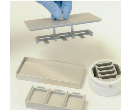
1 The cryomould kit (optional) allows to carry out standardized flash freezing.
