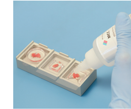
3 Fill the cryomould with the Milestone MCC compound.
