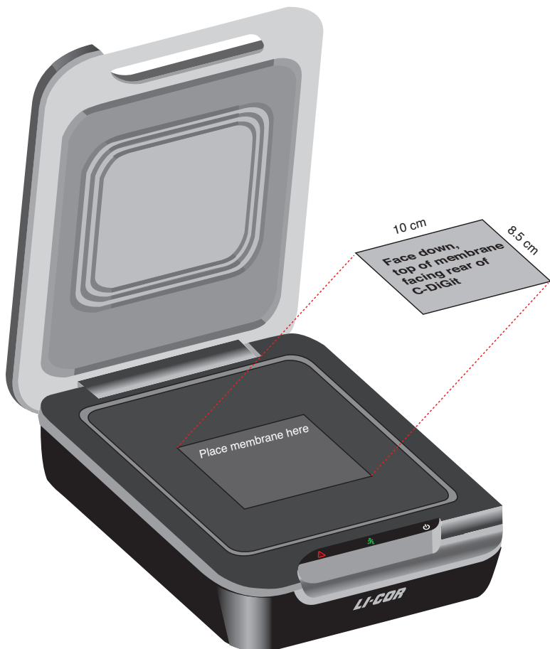
Figure 3-4. The imaging surface is designed to scan a single membrane up to 10 cm x 8.5 cm.
