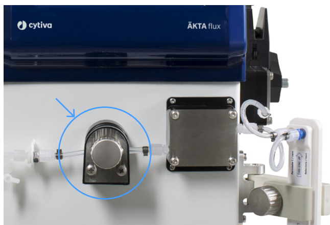
Fig 3. Retentate pressure control valve.
