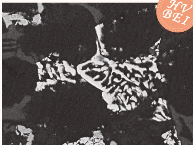
Sample: Aluminum alloy 10 \mu\text{m} Backscattered electron image Accelerating voltage 10 kV, magnification 3,000x
