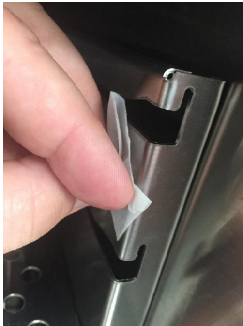
Figure 17 - Cleaning Surface for Sensor Adhesion
