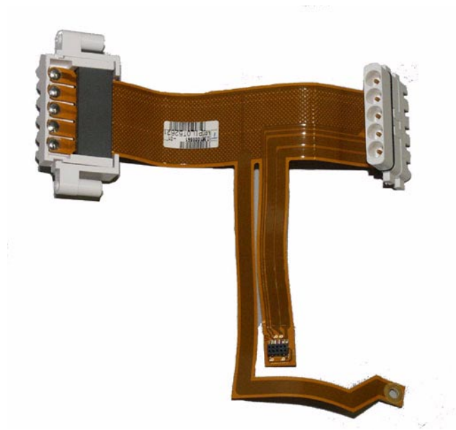
Figure 7 Module bus flex board
