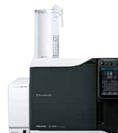
EGA/PY-3030D Pyrolyzer (Frontier Laboratories)
