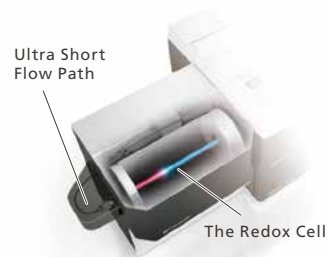
Sulfur Chemiluminescence Detector (SCD-2030)
