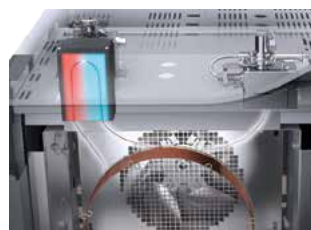
Flame Ionization Detector (FID-2030)
