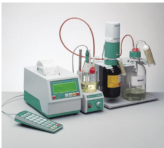
756 KF Coulometer with 700 Dosino for automatically aspirating the titration vessel contents and adding fresh reagent. Dosino and waste bottle are mounted on the 6.2055.100 bottle support.
